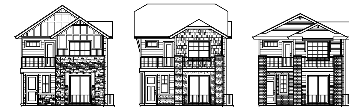
SFD TUCKUNDER PLAN 4 - FRONT ELEVATION - 'D' SFD TUCKUNDER PLAN 4 - FRONT ELEVATION - 'E' SFD TUCKUNDER PLAN 4 - FRONT ELEVATION - 'F'
