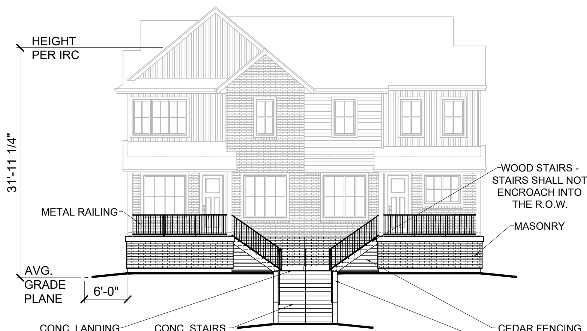
GRADE SEPARATED ELEVATION - FRONT ELEVATION STYLE 'D' SHOWN, ALL PLANS & ELEVATIONS SIMILAR SCALE: 1/8" = 1'-0"
