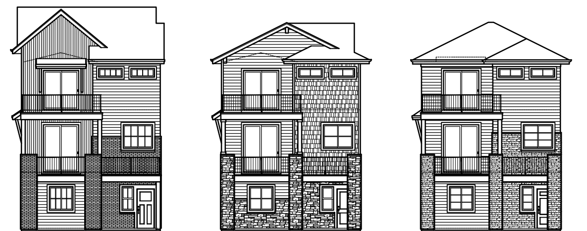
SFD 3-STORY PLAN 1 - FRONT ELEVATION - 'D' SFD 3-STORY PLAN 1 - FRONT ELEVATION - 'E' SFD 3-STORY PLAN 1 - FRONT ELEVATION - 'F'
