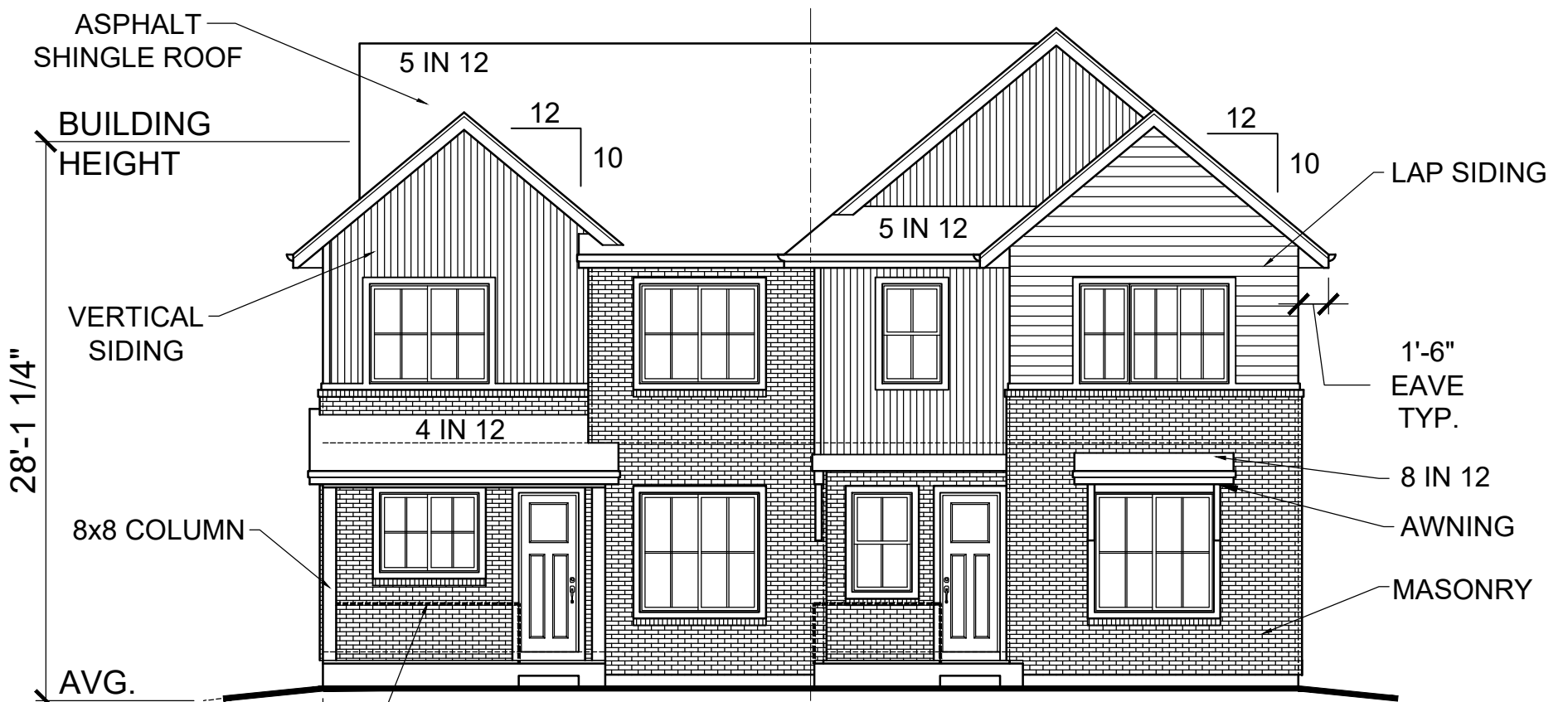
PLAN 2 & 3 ELEVATION 'D' - FRONT 53% MASONRY PROVIDED AT FRONT SCALE: 1/8" = 1'-0" 51% MASONRY AVERAGE TOTAL (50% REQ.) GUARDRAIL WHEN PORCH RISES 30" OR HIGHER ABOVE GRADE
