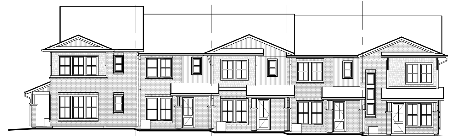
3 5-PLEX-A - FRONT ELEVATION - SHINGLE STREETSCAPE 1/16" = 1'-0"
